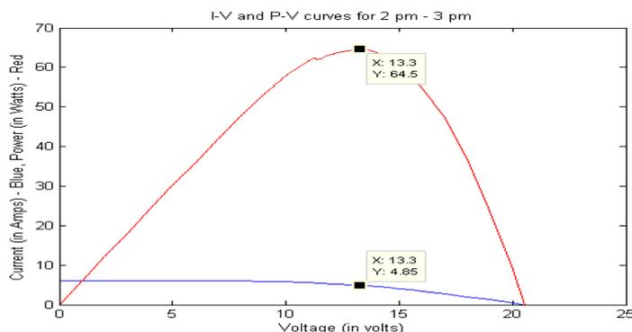
Fig. 5 P-V characteristics of a PV system
