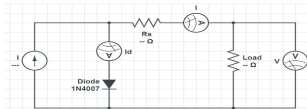
Fig. 3 Simplified general equivalent circuit for a solar cell
